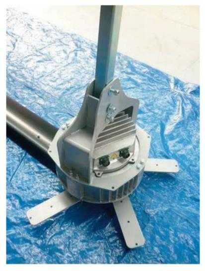
PLACE ROD INTO MOTOR HOLDER AND FIX WITH SCREWS, NUTS AND BOLTS
