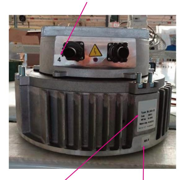
Motoinverter type and Serial Number label Inverter parameterization Blades Diameter Set label
