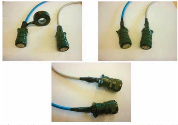
IT'S MANDATORY TO PROTECT THE BACK PART OF CONNECTORS FROM HUMIDITY OR DIRT USING INSULATING COIL OR SOME OTHER MATERIAL THERMALLY SHRINKABLE
