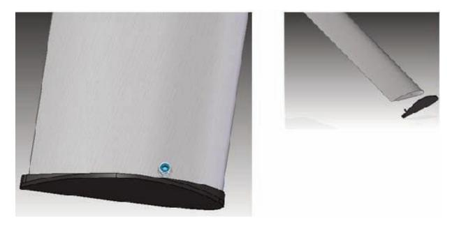
Loosen the screw fissing the plastic Winglet to the blade
