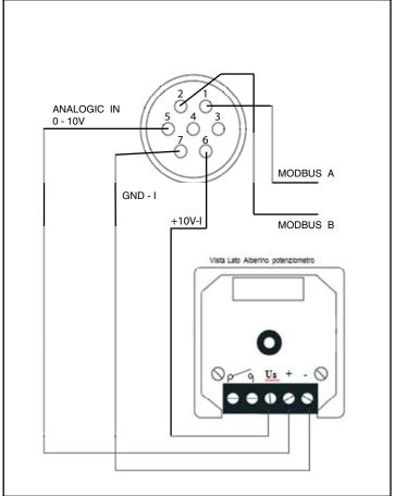
Electric Scheme - Option 2: External Potentiometer with DIN box Vortice code: 12828
