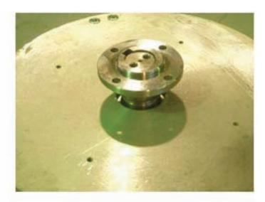
AFTER DISASSEMBLED BLADE SUPPORT, DISASSEM-BLY HUB
