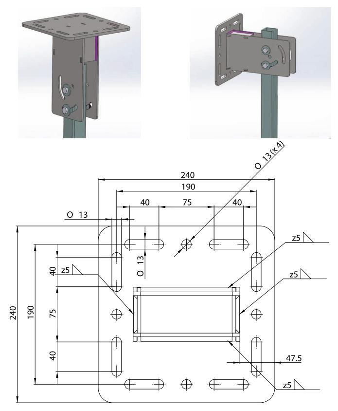
PLACE ROD INTO ROD HOLDER AND FIX WITH SCREW, NUTS AND BOLTS ASSEMBLY POSITION FOR ROD HOLDER DEPENDS ON INSTALLATION STUDY AND DESIGN
