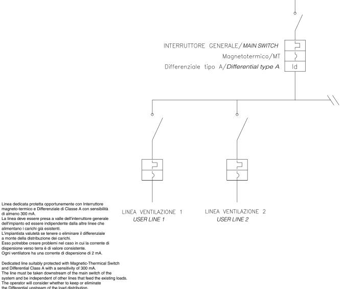
the Differential upstream of the load distribution. It could create problems in the case where the leakage
